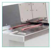
Self-adjusting feeder mechanism enables a wide variety of envelopes to be processed with no tamping or jogging required.
